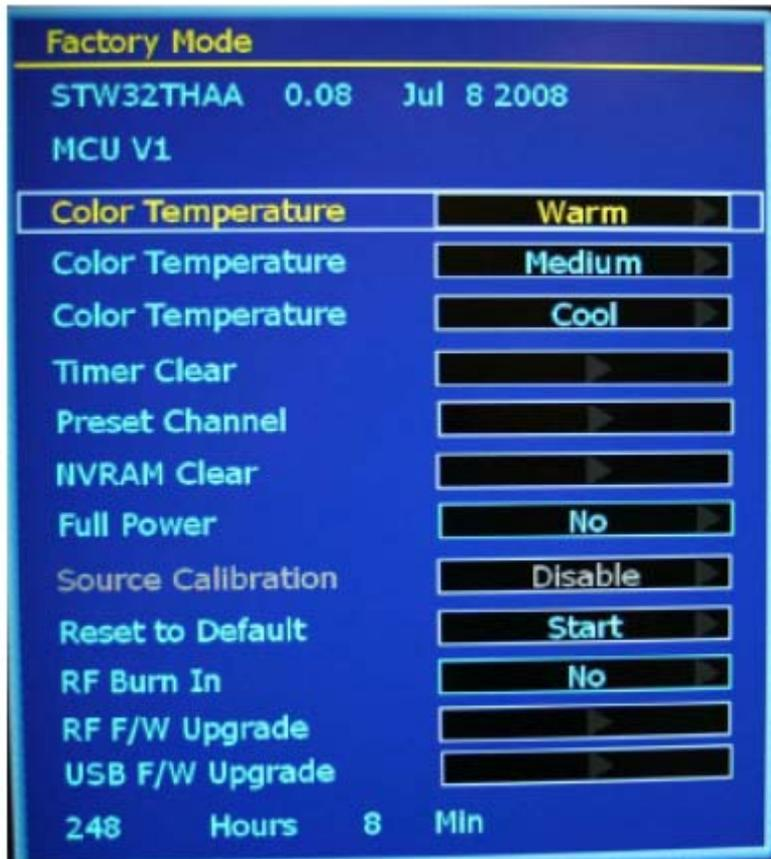
To enter the factory mode, you must press “Left Arrow (<), then Exit, then Enter” within approximately two seconds. To end this function, press exit or simply turn the television off.
